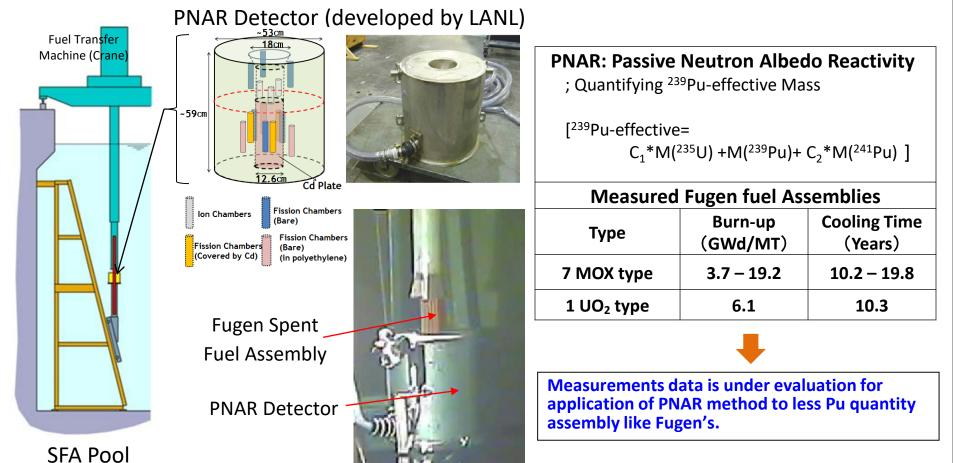
PNAR detector developed by LANL was installed by JAEA in the Fugen spent fuel pool. Measurements / transfers of assemblies were done jointly.
