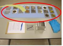
Au, W, Rh, Cu, Co, Mn samples (plates) with different thicknesses were prepared .
